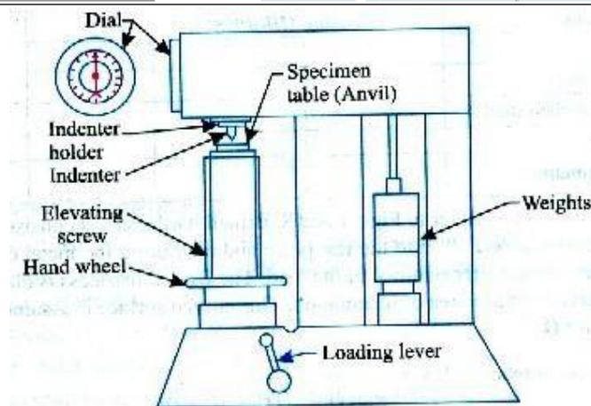
**THEORY:** The hardness of a material is resistance to penetration under a localized pressure or resistance to abrasion. Hardness tests provide an accurate, rapid and economical way of determining the resistance of materials to deformation. There are three general types of hardness measurements depending upon the manner in which the test is conducted:
